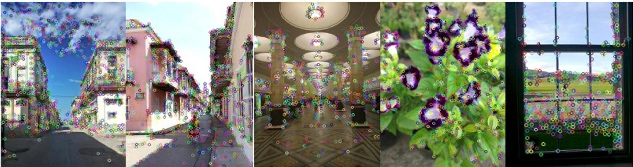
Fig. 15. Results of the feature extraction step made by Shi-Tomasi detector in RGB images.
