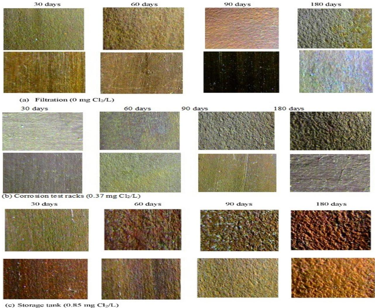
Fig. 9. Image of corrosion of the copper coupons
