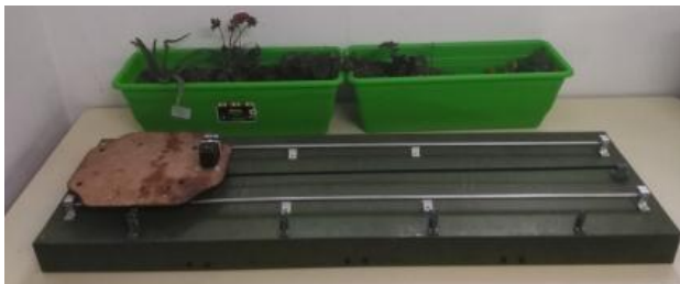
Fig. 8. Translation mechanism for the robot. Architecture of the teleoperation system
