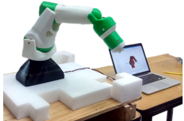
Fig. 6. Implementation of the 5 GDL anthropomorphic robot.
