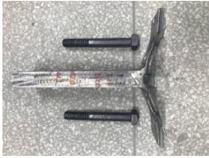
(a) Failure Mode 1: Deformation of the specimens and the finite element model
