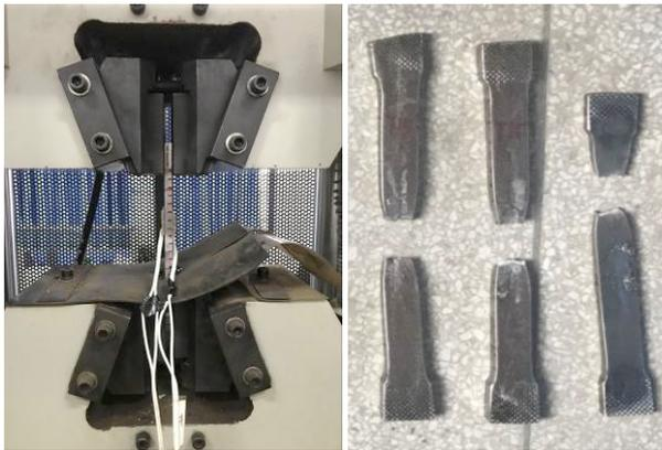
Fig. 2. Loading device for the tensile test and the morphologies of the specimens after failure
