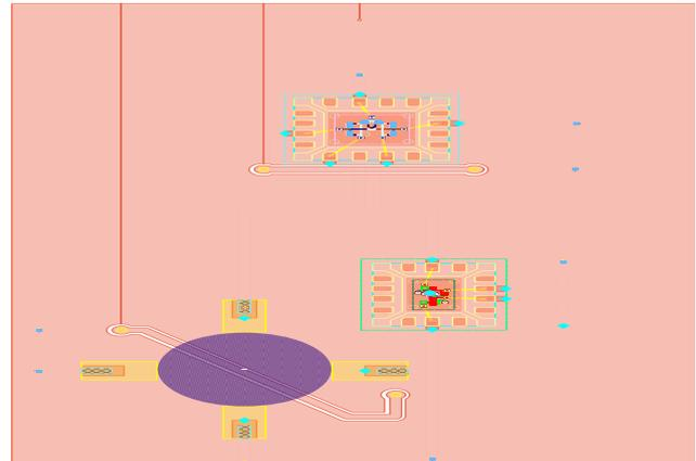
Fig. 11. RF board level smart antenna transceiver system layout [89].
