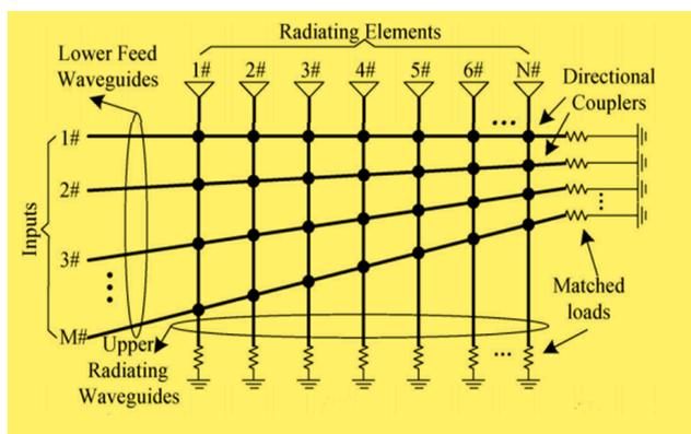
Fig. 3. Schematic of a Blass matrix [71].
