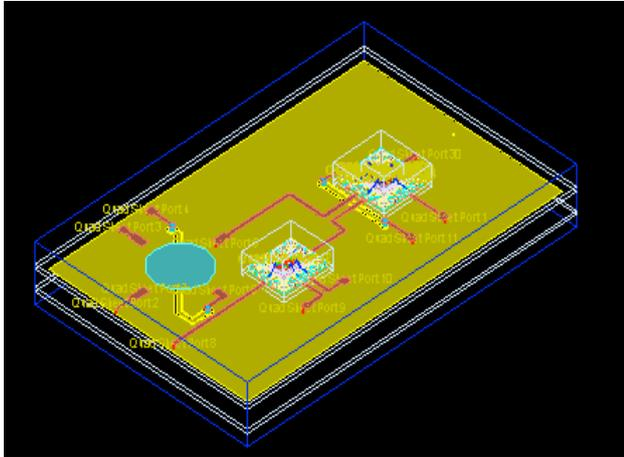
Fig. 12. Isometric 3D EM Preview of the designed Antenna [89].
