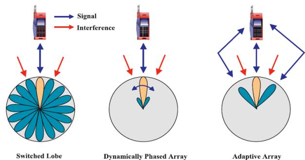
Fig. 5. Different smart antenna concepts [91].
