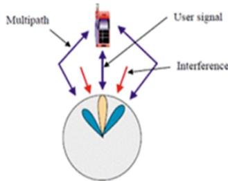
Fig. 8. Adaptive/smart antenna array [91].
