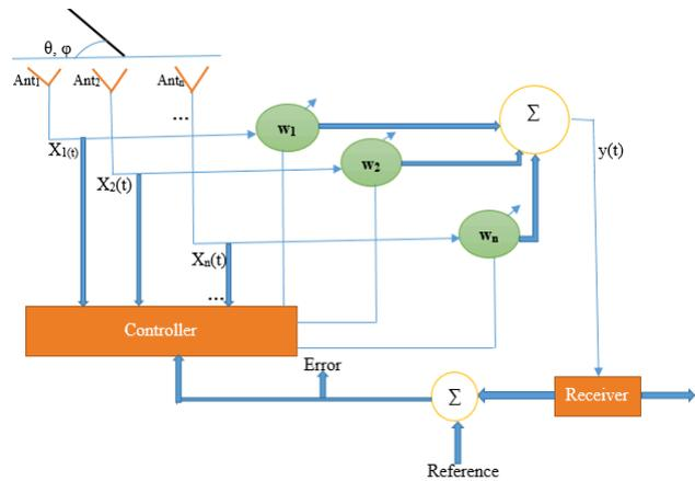
Fig. 7. Basic layout for adaptive antenna array.
