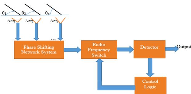
Fig. 1. Block diagram of a switched-beam antenna structures.
