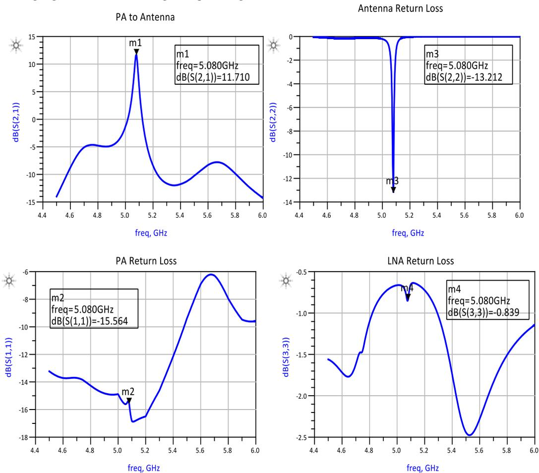
Fig. 13. Results of RF transceiver antenna [89].
