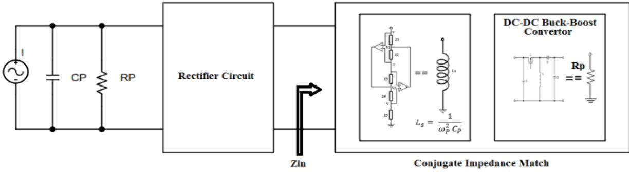
Fig. 9. Proposed Complex conjugate impedance matching.
