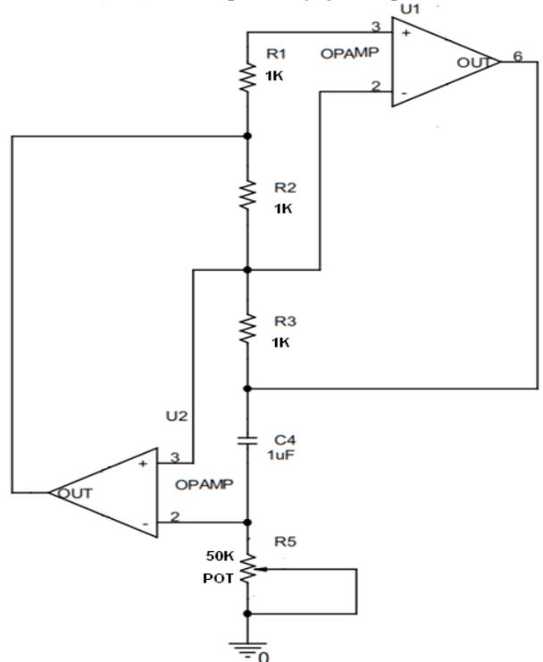
Fig. 11. Proposed Antoniou inductor simulation circuit for complex conjugate impedance matching.
