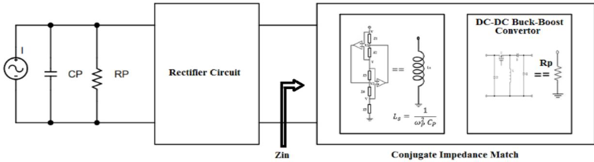
Fig. 9. Proposed Complex conjugate impedance matching.
