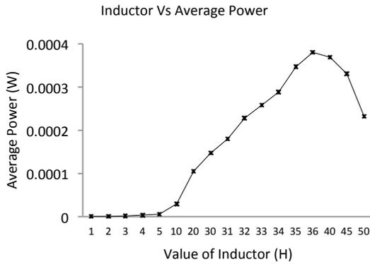
**Fig.12.** Graph plotted between Proposed Antoniou inductor simulation circuit for complex conjugate impedance matching and Average power.
