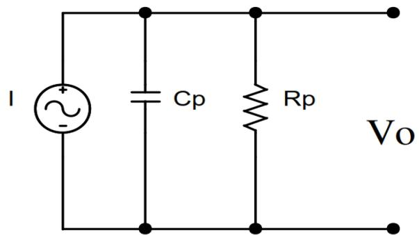
Fig. 1. Equivalent circuit model of piezoelectric transducer.
