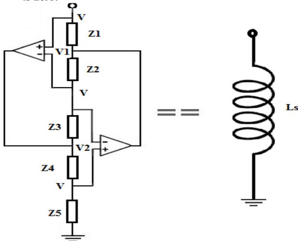
Fig. 10. Proposed op-amp based GIC (Generalized Impedance Converter).
