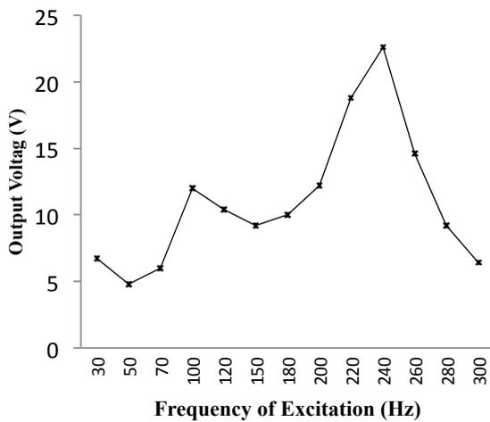
**Fig. 3.** Measured plot of output voltage at various excitation frequencies (Hz) for Q220-A4-203YB piezoelectric transducer.
