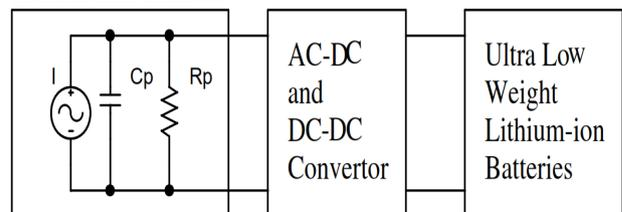
Fig. 2. Block implementation of Piezoelectric Harvester to charge ultra-low power lithium-ion batteries
