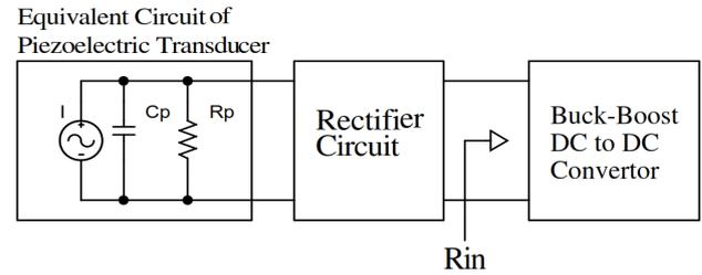
**Fig. 4.** Block Diagram of Resistive Impedance Matching Circuit for Piezoelectric Energy Harvesting
