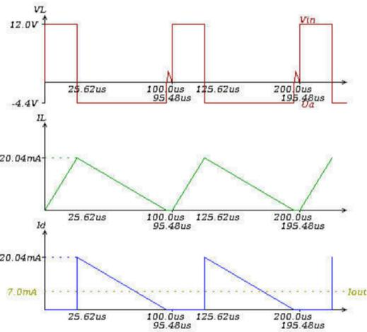
**Fig. 8.** Obtained Waveforms for Buck- Boost Converter.
