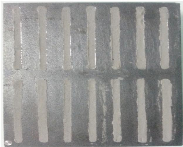
**Fig. 2.** Preset of the cladding powder
