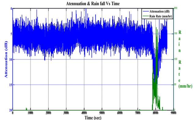
Fig. 5. Rain rate and Attenuation w.r.t Time
