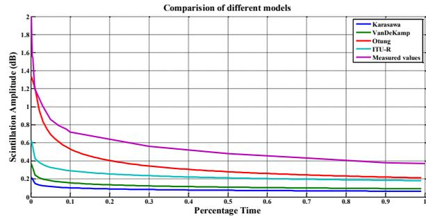
Fig. 9. Comparison of different models with measured scintillation.
