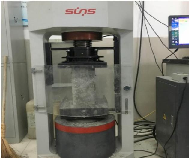
**Fig. 1.** Pressure testing machine at 5000 kN
