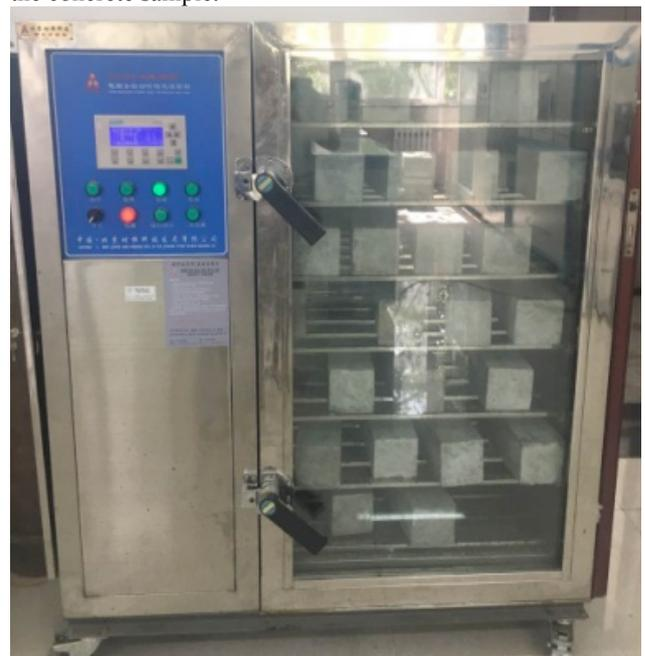
**Fig. 3.** Carbonation test chamber
