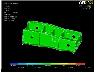
**Fig. 7.** Stresses in Y directions  $(S_y)$  of composite foundation
