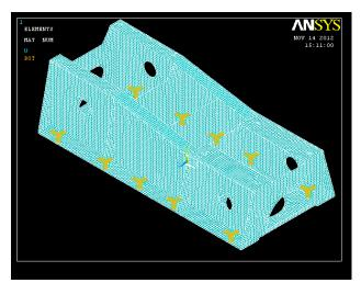
Fig. 2. Fixed boundary condition of foundation
