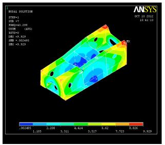
Fig. 9. 7th mode shape of CNT reinforced with CFRP foundation (Free-Free Eigen value analysis
