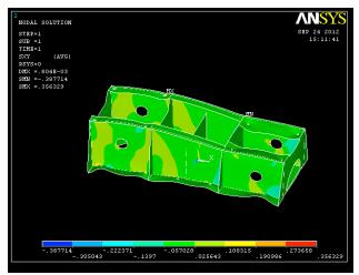
Fig. 8. Shear stresses in XY directions  $(S_{xy})$  of composite foundation
