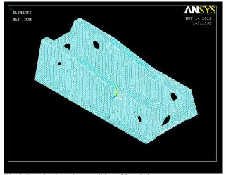
Fig. 3. Free-free boundary condition of foundation
