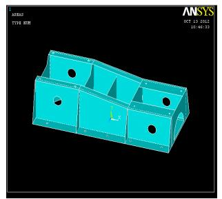
Fig. 1. Shell model of foundation
