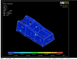
Fig, 4. Displacement and von-mises stress of mild steel foundation
