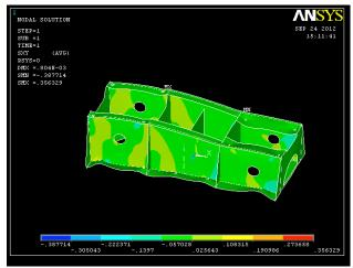
Fig. 6. Stresses in X directions (Sx) of composite foundation
