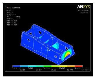
Fig 5. 15th mode shape of mild steel foundation (free -free boundary condition)
