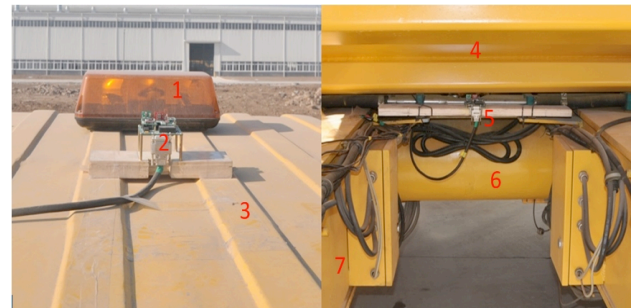
1—Top warning light of the front frame, 2—Inertial navigation module of the front frame, 3—Cab top cover, 4—Body, 5—Inertial navigation module of the rear frame, 6—Torsion tube of the rear frame, 7—Left longitudinal beam of the rear frame Fig. 7. Installation position of the inertial navigation module of the front and rear frames
