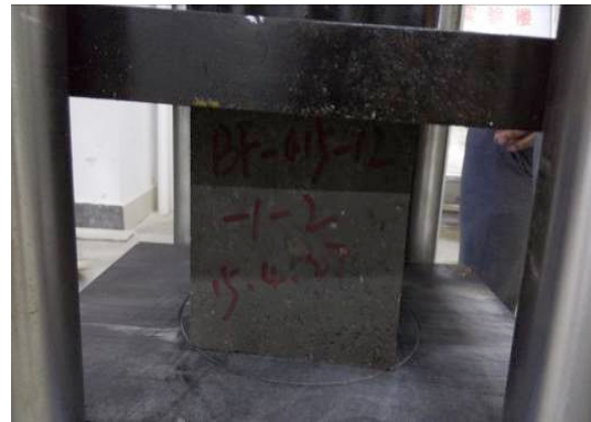
Fig. 3. Cube compressive strength test of specimen
