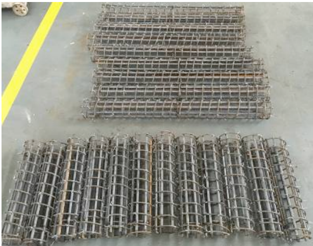
Fig. 4. Reinforcing steel bars for short test columns
