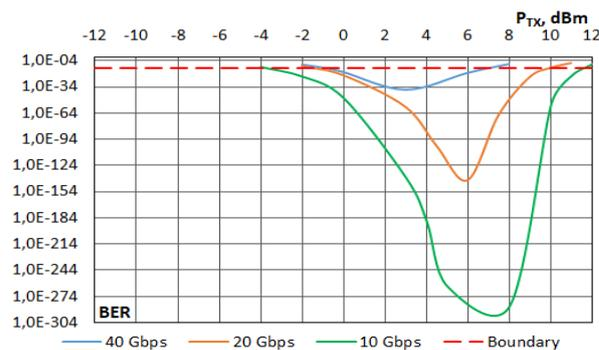
Fig 9. BER characteristics for CSRZ modulated optical signal
