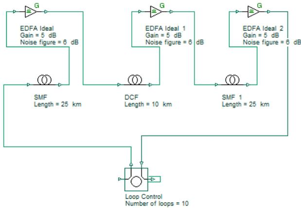
Fig 5. Transmission channel model with symmetrical DCS
