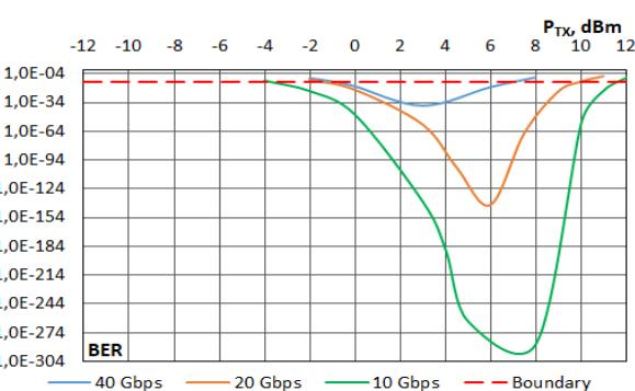
Fig 9. BER characteristics for CSRZ modulated optical signal
