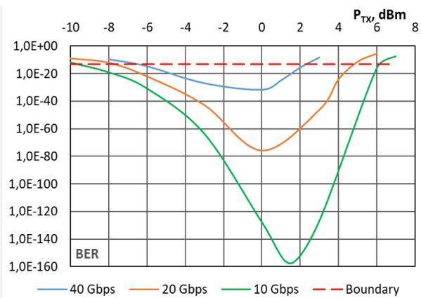
Fig 7. BER characteristics for NRZ modulated optical signal
