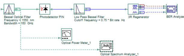
Fig 6. Optical receiver model
