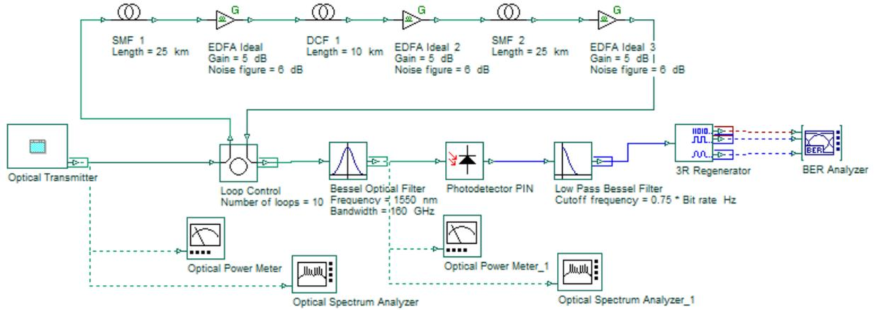
Fig. 1. Proposed model for simulation of single-channel optical communication line with symmetrical DCS
