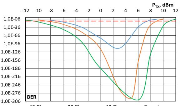
Fig 8. BER characteristics for RZ modulated optical signal
