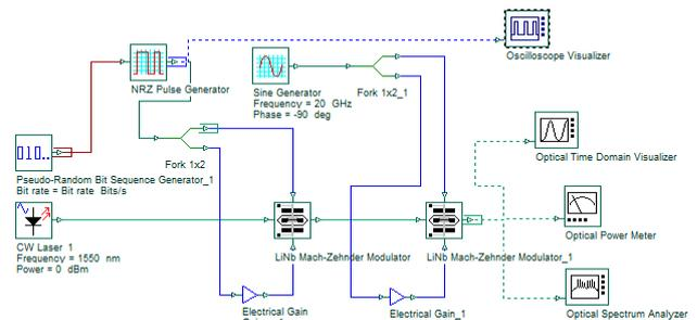
Fig. 4. Model of externally CSRZ modulated optical transmitter
