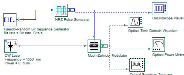
Fig. 2. Model of externally NRZ modulated optical transmitter
