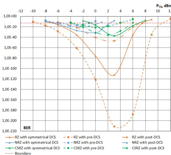
**Fig. 10.** Comparative analysis of BER characteristics for different dispersion compensation schemes at 40 Gbps
