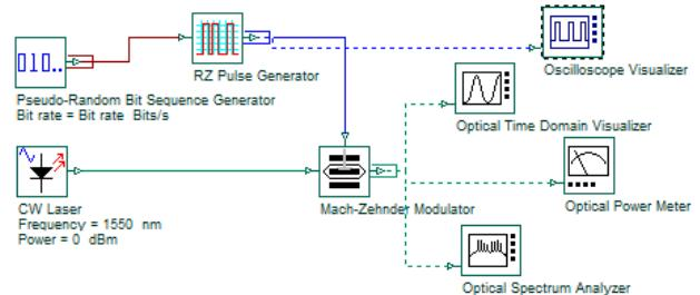
Fig. 3. Model of externally RZ modulated optical transmitter
