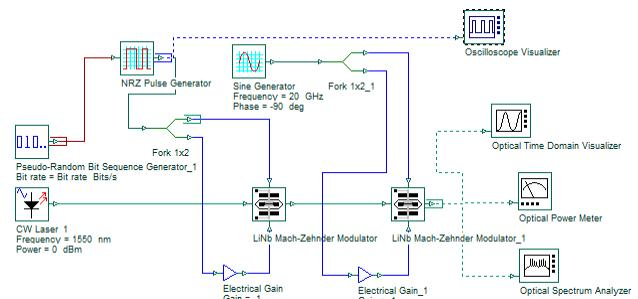
Fig. 4. Model of externally CSRZ modulated optical transmitter
