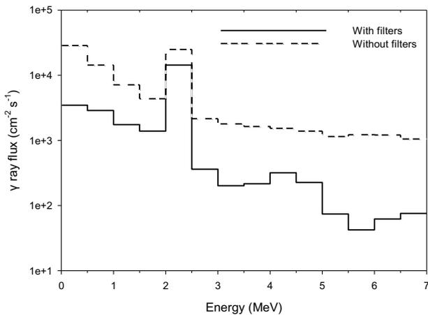
**Fig 2.** The  $\gamma$  ray energy spectra at the exit of the system with and without the beam filters.
