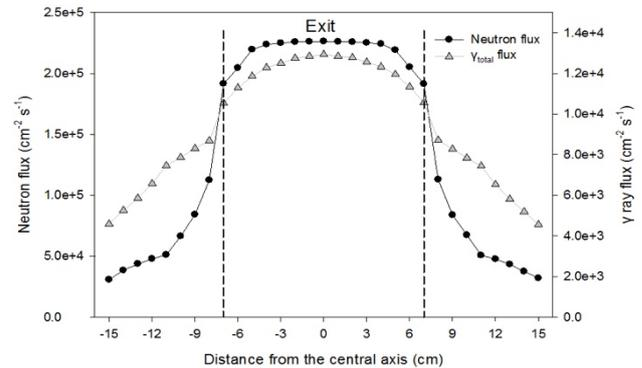
**Fig 4.** Neutron and  $\gamma_{total}$  fluxes on a perpendicular plane at the head position.
