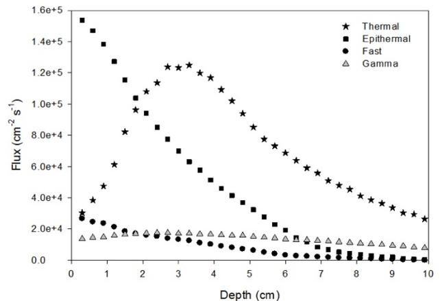
**Fig 5.** Distribution of the neutron and  $\gamma_{total}$  fluxes on the head phantom.
