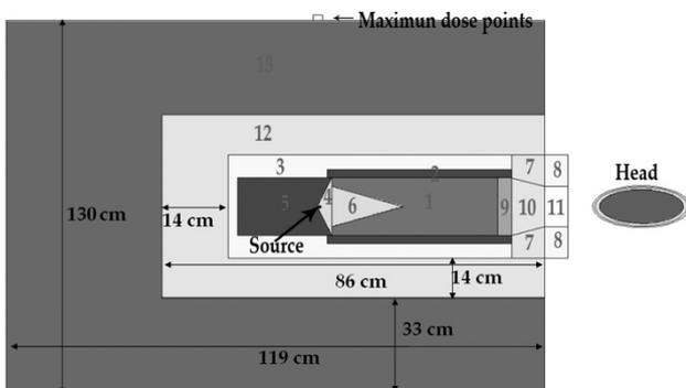
**Fig 1.** Geometric configuration of the BNCT system. (1) Fluental, (2) nickel reflector (3) graphite reflector, (4)  $\text{D}_2\text{O}$  collimator (5) nickel reflector, (6)  $\text{D}_2\text{O}$ , (7) bismuth, (8) borated lithium, (9) titanium as fast neutron filter, (10) bismuth as  $\gamma$ -ray filter, (11) void, (12) bismuth, (13) borated poly.
