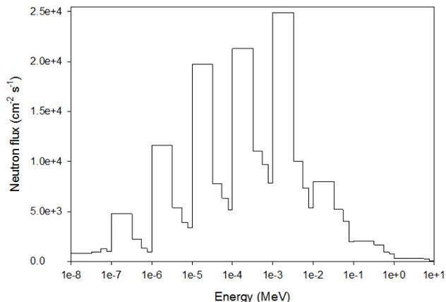
**Fig 3.** Neutron energy spectrum at exit of the facility.
