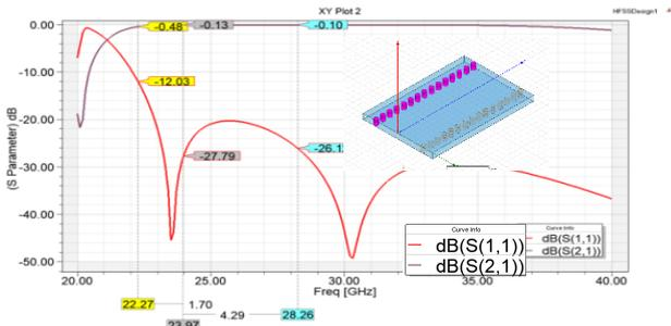
Fig 3. S Parameter (S<sub>11</sub>,S<sub>21</sub>) SIW structure
