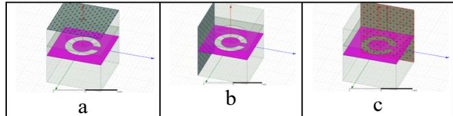
Fig 4. Set boundaries on structure a) Perfect E perpendicular to resonator b) Perfect H side walls and c) set wave port.
