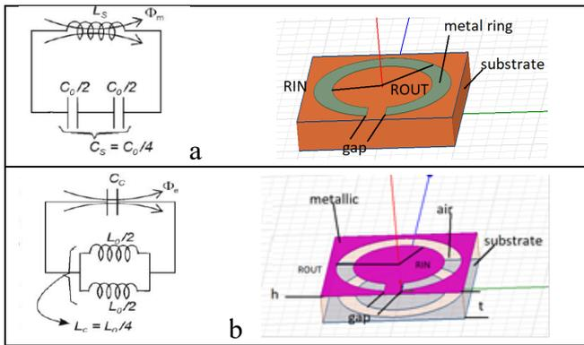
Fig 2.a) Equivalent circuit and design structure a)BC-SRR b) BC-CSRR
