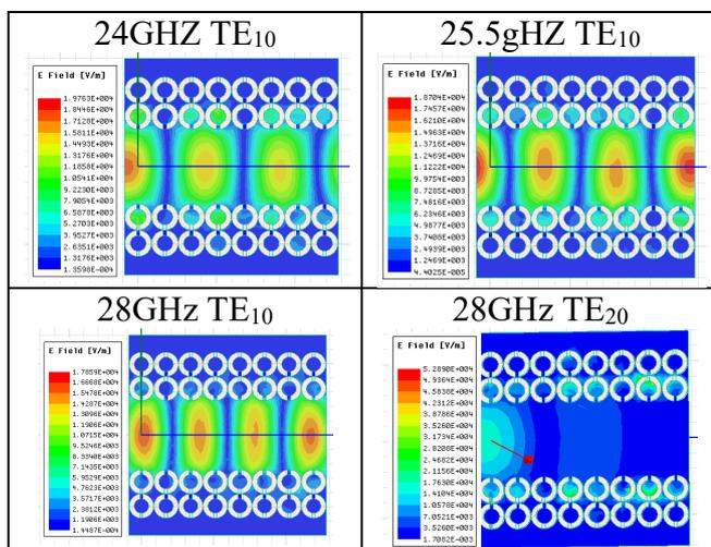
Fig 7. Electric field for three frequency band  $TE_{10}$  mode for a,b,c and  $TE_{20}$  mode for max frequency.
