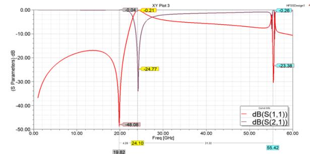
Fig 5. Scattering Parameter (S<sub>11</sub>, S<sub>21</sub>) single BC-CSRR structure.
