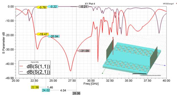
Fig 6. S Parameters  $S_{11}$  red line,  $S_{21}$  dark line of SIW-CSRR structure
