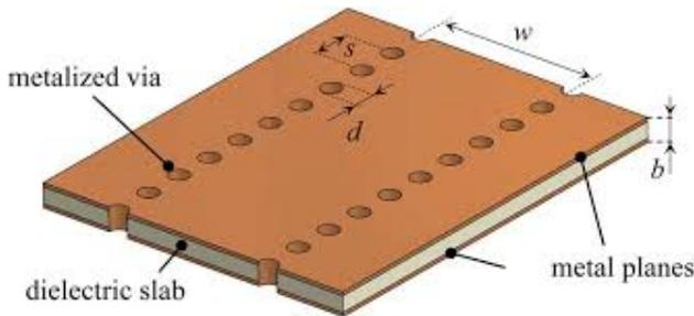
Fig 1.General geometry of SIW [12] .
